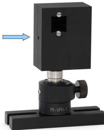
Figure 24: 4-quadrant-diode. The arrow points to the potentiometer for intensity variation (Please use a screwdriver)
