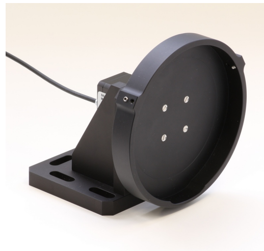
Figure 10: P4S30 with 4" adapter on stiff mount
