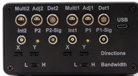
Figure 36: Right panel with additional “Adjust-in” inputs for x and y position of two PSDs
