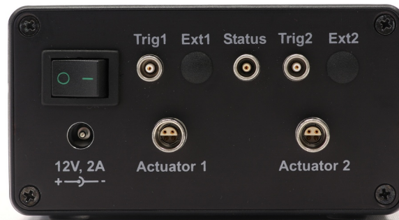
Figure 27: Left panel of controller box with trigger inputs
