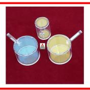
Ultra-High-Vacuum Cell of Drum-Type 鼓形超真空腔
