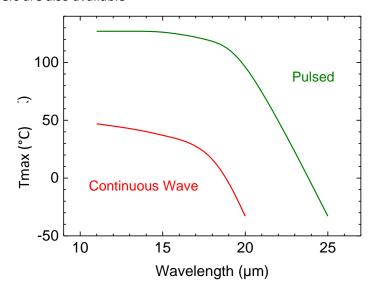
The red curve indicates the maximum chip temperature as a function of the wavelength for CW lasers and the green curve indicates the maximum chip temperature as a function of the wavelength for the pulsed laser.
