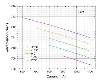
The curves indicate the typical laser singlemode emission wavelength as a function of the applied DC current and laser chip temperature. Lasers with slightly shifted wavelength are also available.
