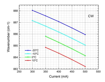
The curves indicate the laser singlemode emission wavelength as a function of the applied DC current and laser chip temperature. Lasers with slightly shifted wavelength are also available.
