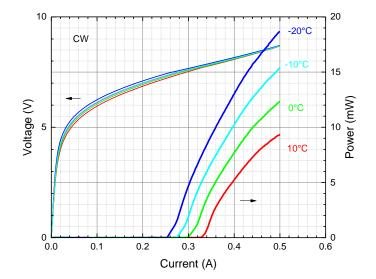
The curves on the left indicate the voltage of the laser as a function of the applied DC current and laser chip temperature.
