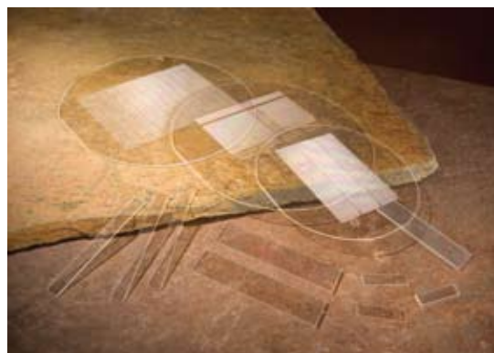
PPLN substrate has been etched to reveal domain strips.
