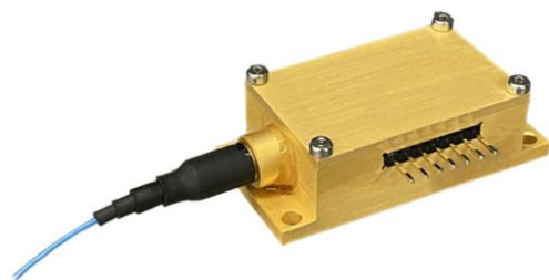
Figure 2. Custom 14-pin butterfly package with PM fiber output
