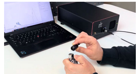
Measuring byproducts of combustion processes with NLIR's MIDWAVE Spectrometer in real time.
