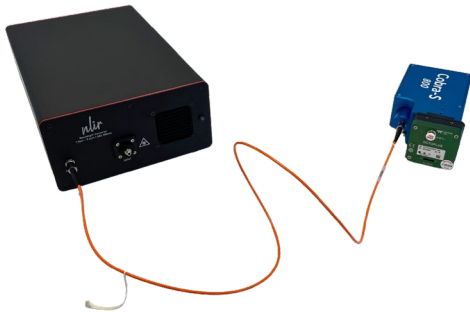
NLIR's SPEKTRUM Wavelength Converter coupled to a 130 kHz Wasatch Photonics Cobra-S OCT Spectrometer.
